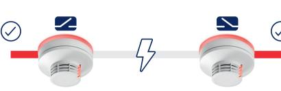
After a short circuit, the loop is re-established from both sides automatically, the short circuit is isolated and the two stubs work without restrictions.
